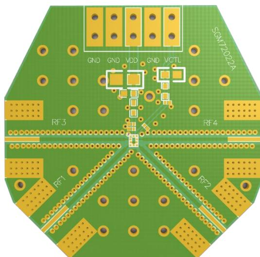
Figure 3. SGM72022A Evaluation Board Layout
