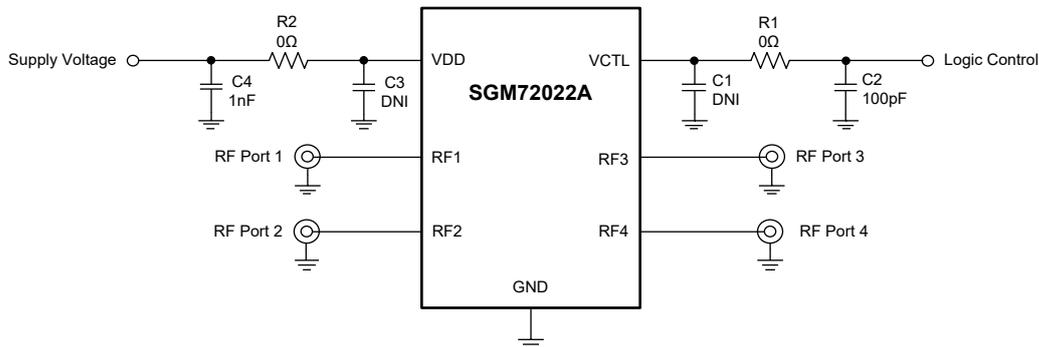
Figure 2. SGM72022A Typical Application Circuit
