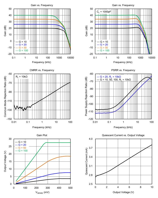
At  $T_A$  = +25°C,  $V_S$  = 12V,  $V_{IN+}$  = 12V, and  $V_{SENSE}$  = 100mV, unless otherwise noted.
