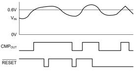
Figure 4. Capability of Latching
