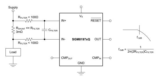
Figure 6. Filtering at the Input (Gain Error: 1.5% to 2.8%)
