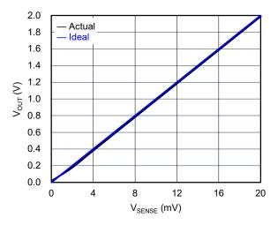
Figure 7.  $V_{OUT}$  vs.  $V_{SENSE}$  for Low  $V_{SENSE}$  Cases 1 and 3 (SGM8197A3Q, Gain = 100)
