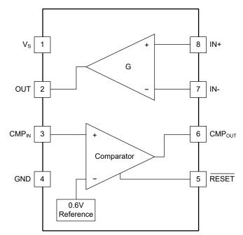
Figure 1. Block Diagram
