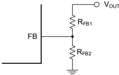
Figure 6. Output Voltage (V<sub>OUT1/2</sub>) Setting
