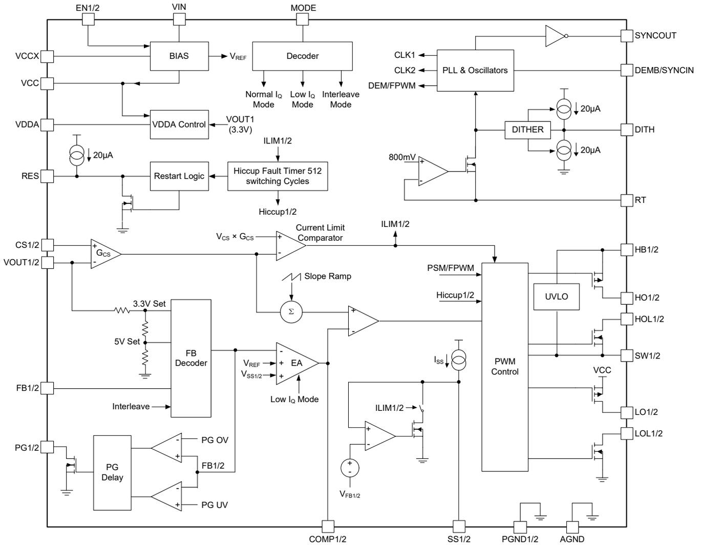
Figure 2. Block Diagram
