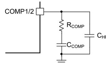
Figure 13. SGM64620 External Compensation
