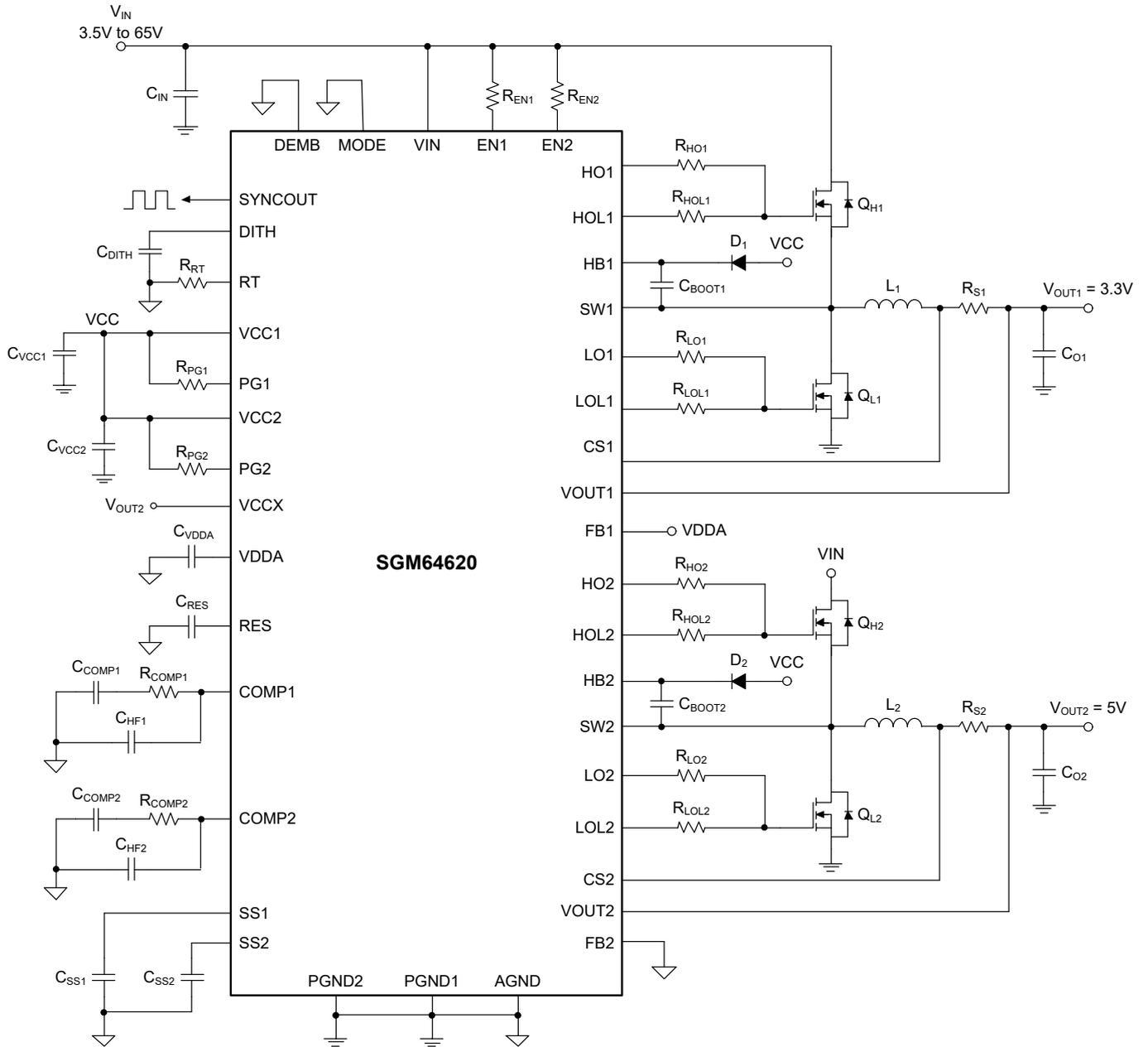
Figure 1. Simplified Schematic
