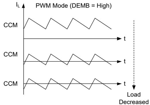
Figure 3. Converter Operation with Forced PWM (PSM Disabled)
