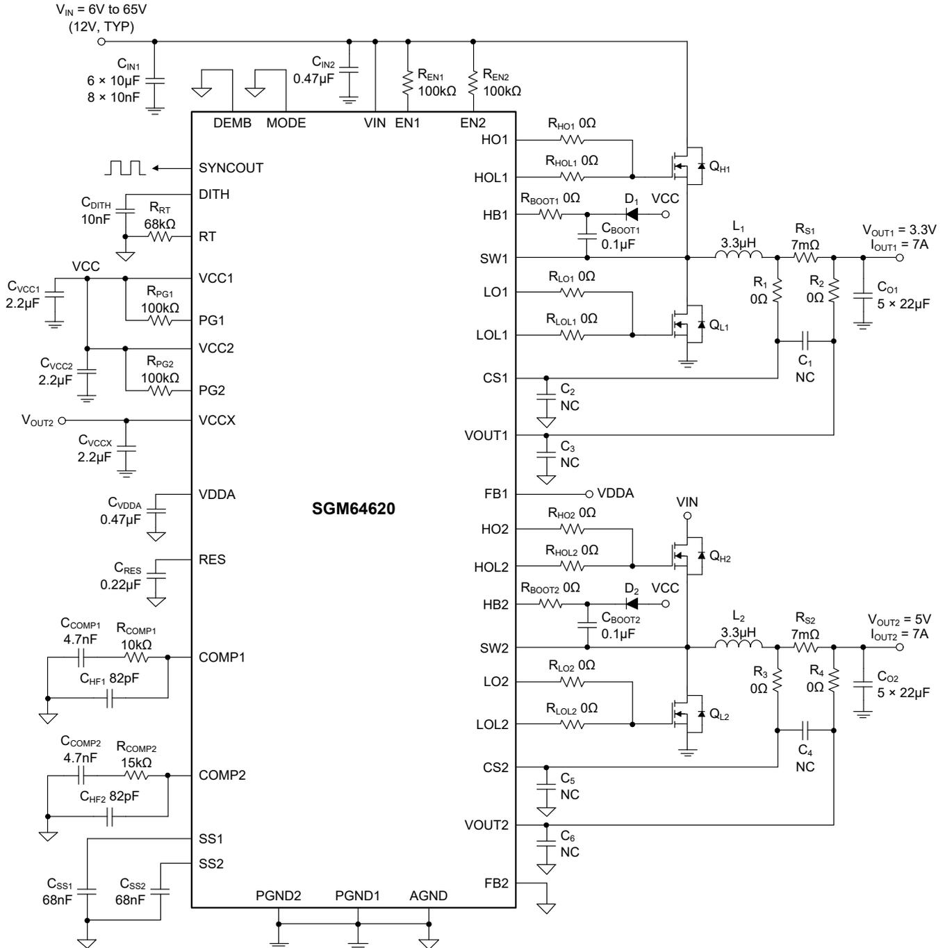
Figure 14. Application Circuit for 3.3V and 5V Dual-Output with 400kHz
