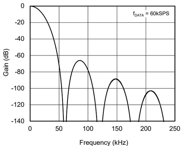
**Figure 8. Frequency Response (Data Rate = 60kSPS)**
