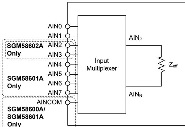
**Figure 6. Analog Input Effective Impedances with Buffer On/Off**
