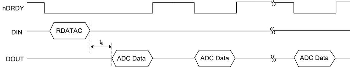
**Figure 14. RDATAAC Command Sequence**
