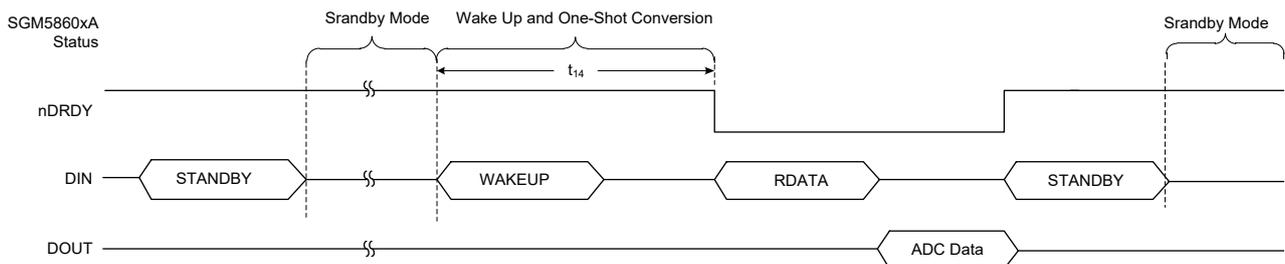
**Figure 13. One-Shot Conversions Using the STANDBY Command**
