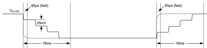
Figure 6. V<sub>ELVSS</sub> Transition Time Control
