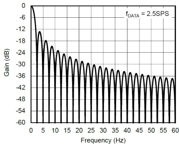
**Figure 9. Frequency Response (Data Rate = 2.5SPS)**
