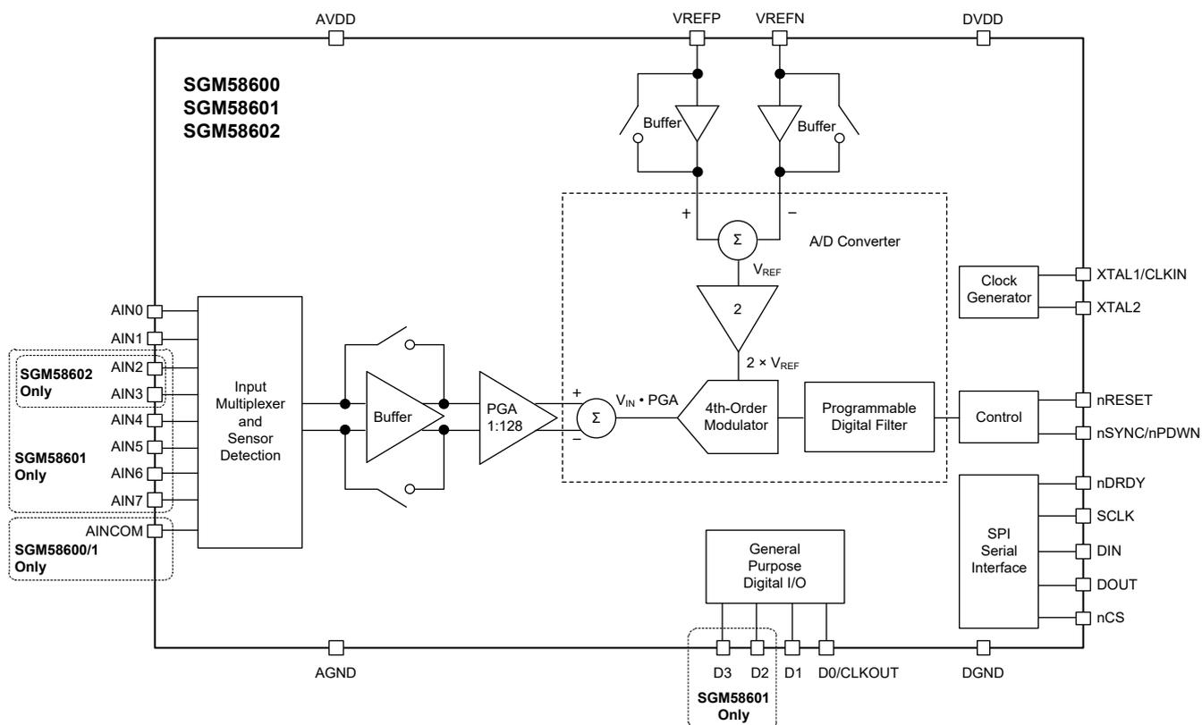
**Figure 4. Block Diagram**
