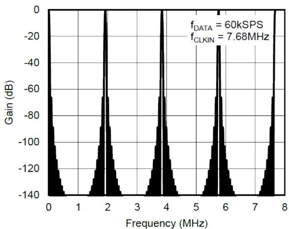
**Figure 10. Frequency Response Out to 7.68MHz (Data Rate = 60kSPS)**
