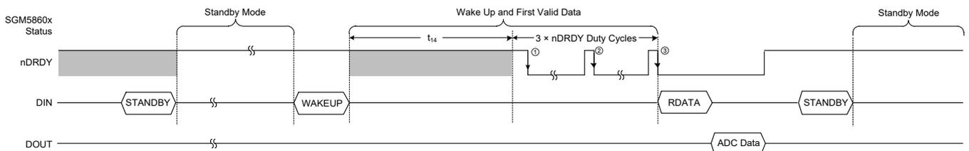
**Figure 13. One-Shot Conversions Using the STANDBY Command**
