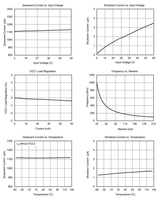
$V_{IN}$  = 24V,  $V_{OUT}$  = 5V, L = 4.7µH, T<sub>A</sub> = +25°C, unless otherwise noted.
