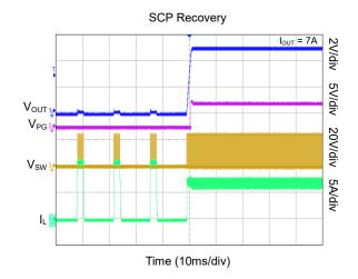
$V_{IN}$  = 24V,  $V_{OUT}$  = 5V, L = 4.7µH, T<sub>A</sub> = +25°C, unless otherwise noted.
