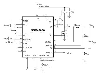
Figure 1. Typical Application Circuit
