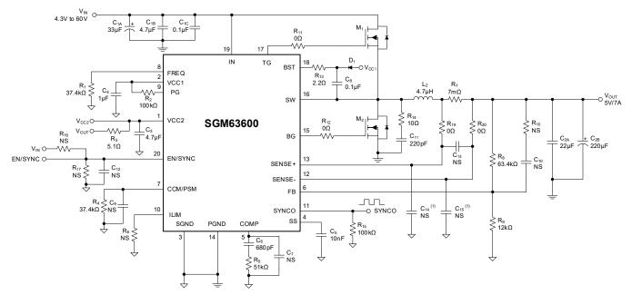
NOTE: 1. The recommended values for  $C_{14}$  and  $C_{15}$  are 10nF in TSSOP package.
