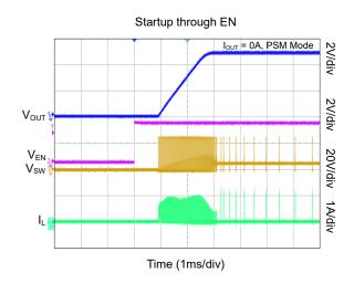
$V_{\text{IN}}$  = 24V,  $V_{\text{OUT}}$  = 5V, L = 4.7  $\mu\text{H},$  T\_A = +25  $^{\circ}\text{C},$  unless otherwise noted.
