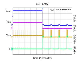
$V_{\text{IN}}$  = 24V,  $V_{\text{OUT}}$  = 5V, L = 4.7  $\mu\text{H},$  T\_A = +25  $^{\circ}\text{C},$  unless otherwise noted.
