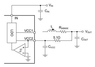
Figure 7. Powering VCC2 from VOUT
