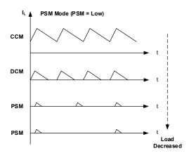
Figure 4. Converter Operation with Forced PWM (PSM disabled) and PSM Enabled (constant or reduced frequency)
