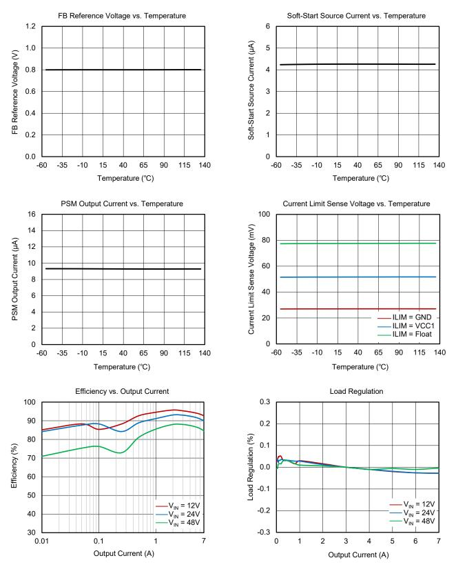
$V_{IN}$  = 24V,  $V_{OUT}$  = 5V, L = 4.7µH, T<sub>A</sub> = +25°C, unless otherwise noted.
