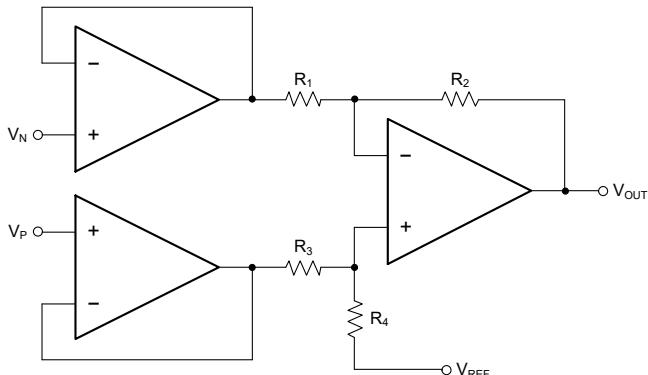
Figure 4. High Input Impedance Difference Amplifier
