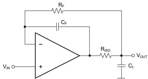
Figure 1. Circuit to Drive Heavy Capacitive Load
